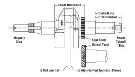
The PTO Extension, the distance from the dashed line to the end of the crankshaft, is measured from:
